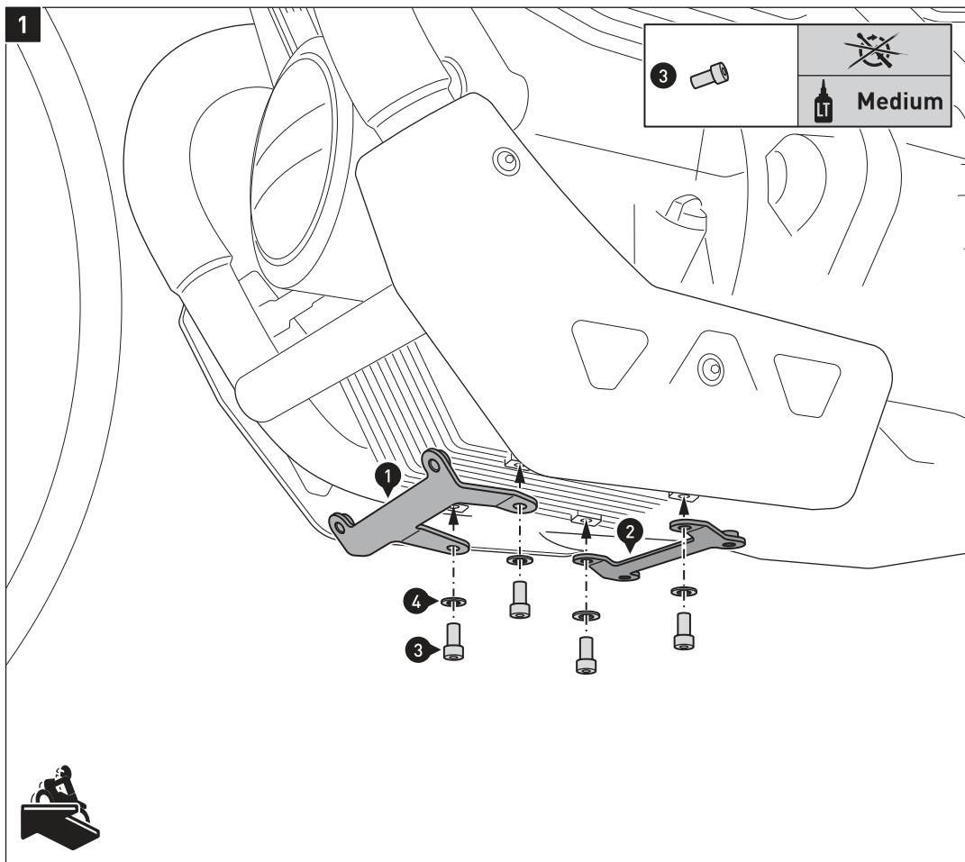
Attach the mounting brackets (1) and (2) to the vehicle, as shown in the drawing.
