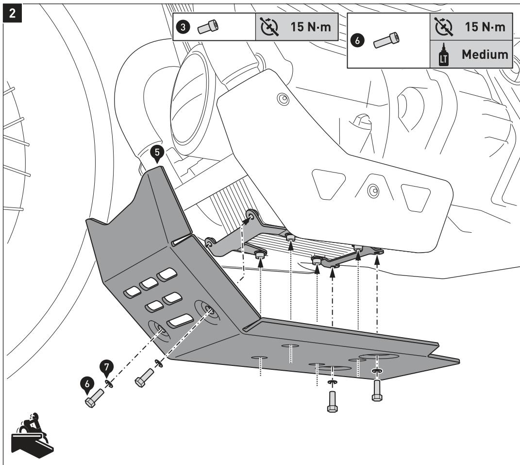
If all parts are positioned without excess tension, tighten the screws as specified.
