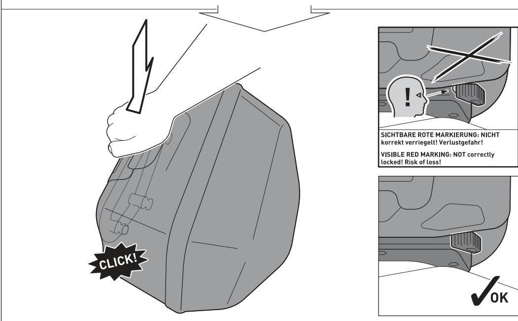
Place the three locking openings of the side case onto the guide bolts of the mounted SLC side carrier. Then press the side case slightly downward, until it properly rests on the SLC side carrier.
