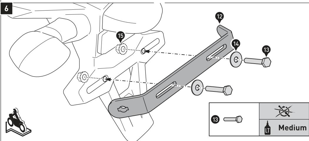
**NOTE:** Follow step [4] & [5] only if the mounting holes of the mudguard do not match with the hole pattern of the crossbar [12].
